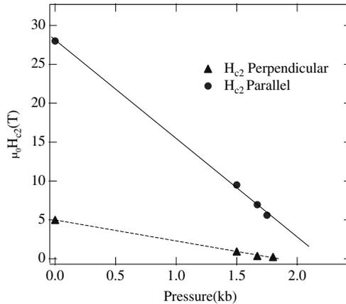
Fig. 2. Pressure dependence of parallel (circles) and perpendicular (triangles) critical field. The error is approximately the size of the symbols. The two ambient pressure points come from Ref. 16.
