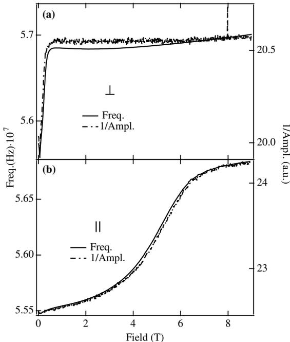
Fig. 1. The rf penetration (proportional to the change in frequency) as a function of magnetic field for the orientation perpendicular to the conducting planes (a) and the parallel orientation (b).  $H_{c2}$  is determined by the intersecting point between the linear extrapolation of the normal state and the superconducting transition.
