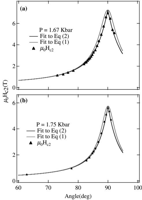
Fig. 4. Angular dependence of  $H_{c2}$  at 1.67 kbar (a), and 1.75 kbar (b). For both graphs, the continuous black line represents a fit with Lawrence–Doniach equation and the gray curve is a fit to the anisotropic 3D Ginzburg–Landau equation.
