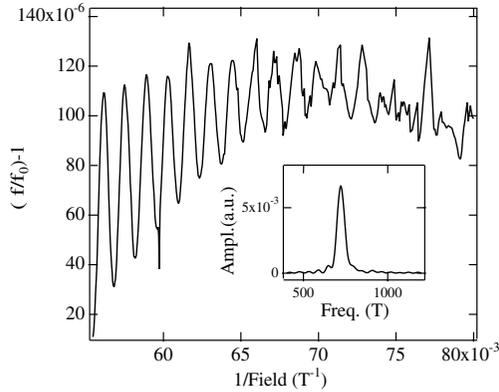
Fig. 5. Magnetoresistance oscillations of  $\kappa$ -(BEDT-TTF) $_2$ Cu(NCS) $_2$  at  $P=1.67$  kbar and  $T=90$  mK. The inset shows the FFT of the oscillations.
