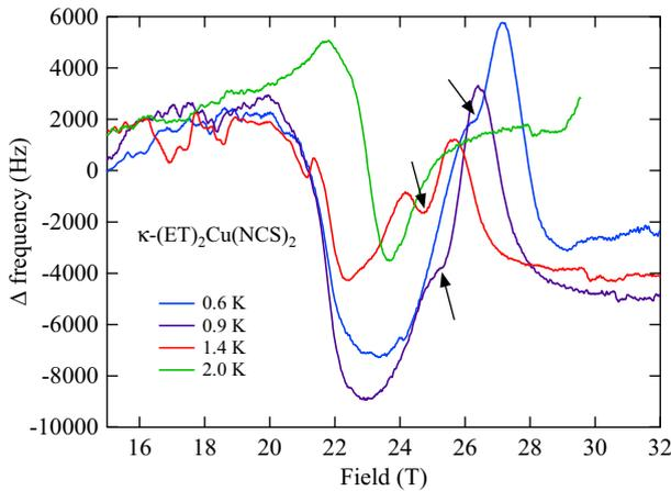
**Fig. 6** Pulsed field sweeps near the entrance to the FFLO phase showing the dip in the penetration depth after a background is subtracted. The large feature develops for all temperatures at about 21 T. A second feature found in all the the sweeps below 2.0 K may be a change in the nature of the FFLO phase and is plotted in the phase diagram in Fig. 3 (Color figure online)
